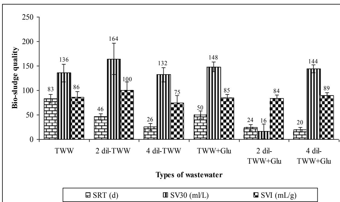
Figure 7. The bio-sludge qualities of SBR system operated with TWW and diluted-TWW+glucose solutions under MLSS of 3,000 mg/L and HRT of 5 days.
