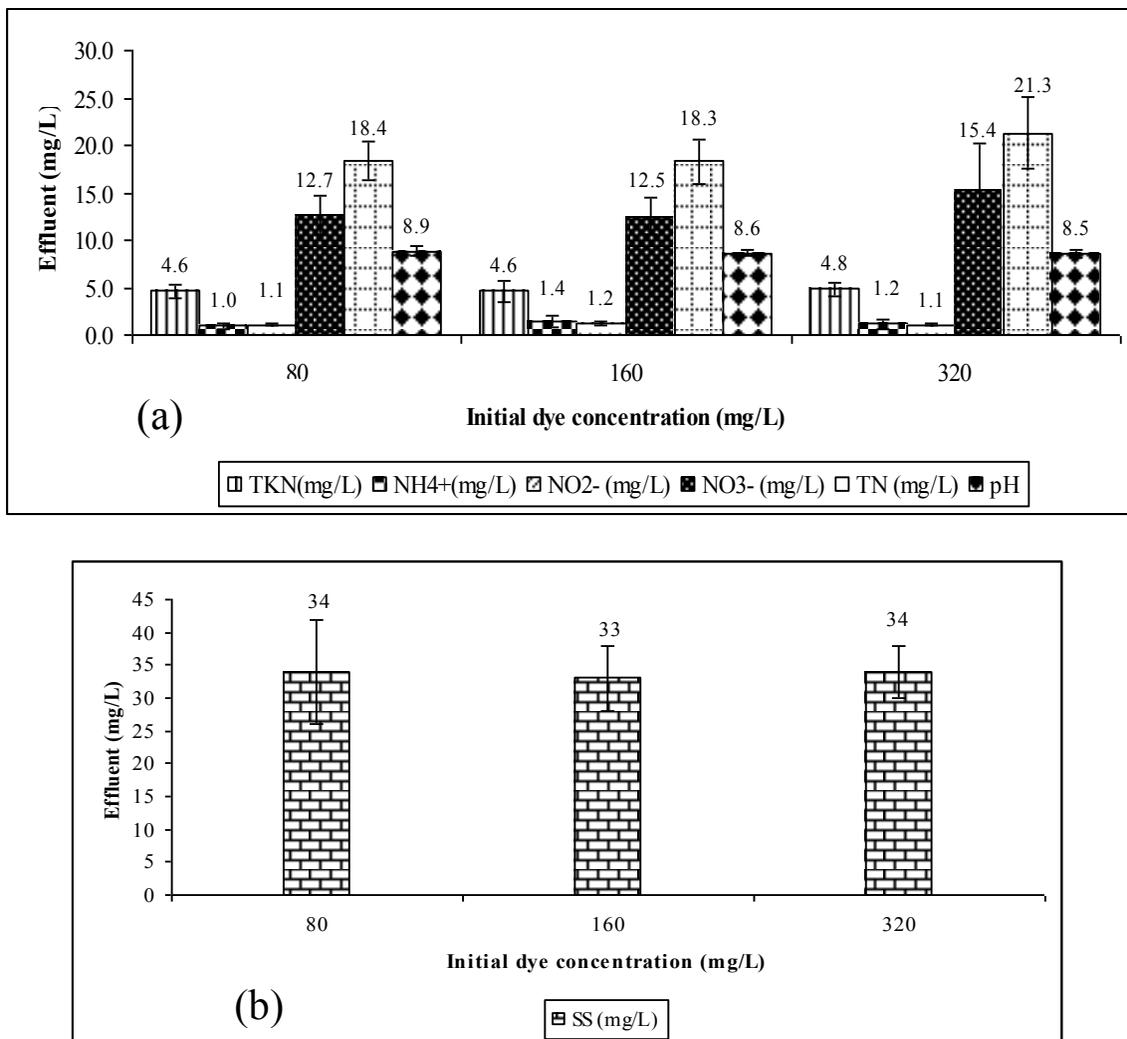
Figure 4. Effluent qualities (a: TKN, NH<sub>4</sub><sup>+</sup>, NO<sub>2</sub><sup>-</sup>, NO<sub>3</sub><sup>-</sup>, TN and pH and b: SS) of SBR system with STWW containing various mixed-disperse dyes (mixture of disperse blue 60 and disperse red 60) concentrations of 80, 160 and 320 mg/L under MLSS of 3,000 mg/L and HRT of 5 days. Remark: Influent TKN = 20.2±3.2 mg/L
