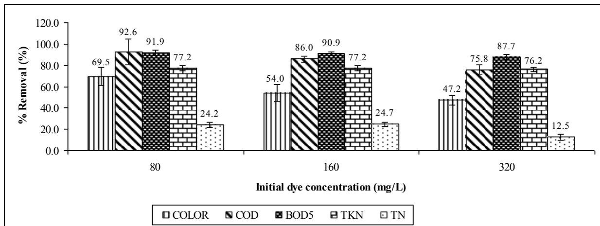
Figure 3. Removal efficiencies of SBR system with STWW containing various mixed-disperse dyes (mixture of disperse blue 60 and disperse red 60) concentrations of 80, 160 and 320 mg/L under MLSS of 3,000 mg/L and HRT of 5 days.
